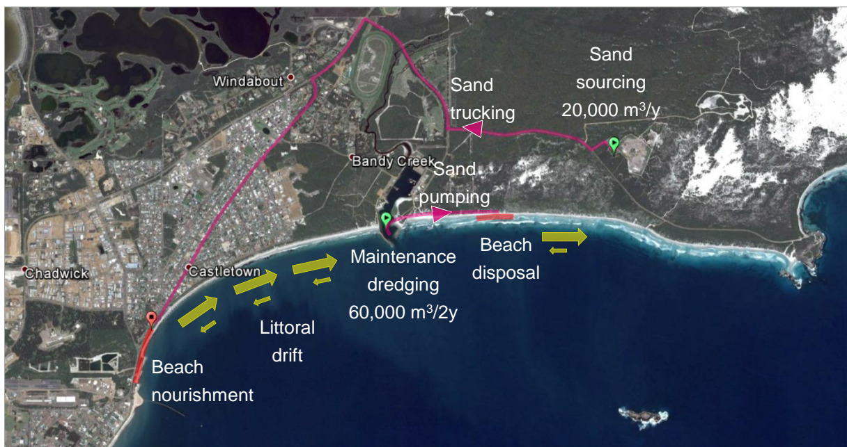
Figure 2-7: Indicative pattern of active sand management in Esperance Bay: Sand “sources” (●), Sand “mechanical” transport (→), beach disposal (-), natural sand drift (→).
