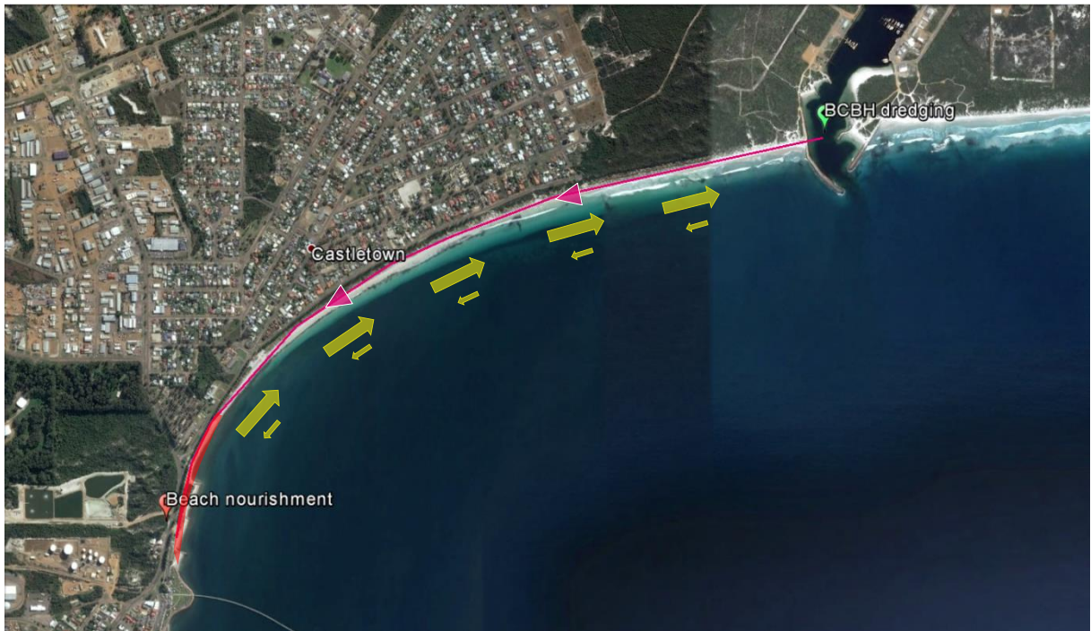
Figure 3-5: Indicative pattern of sand management for coordinated sand back-passing: Sand “sources” (●), Sand ”mechanical” transport (➔), beach disposal (-), natural sand drift (➔).
