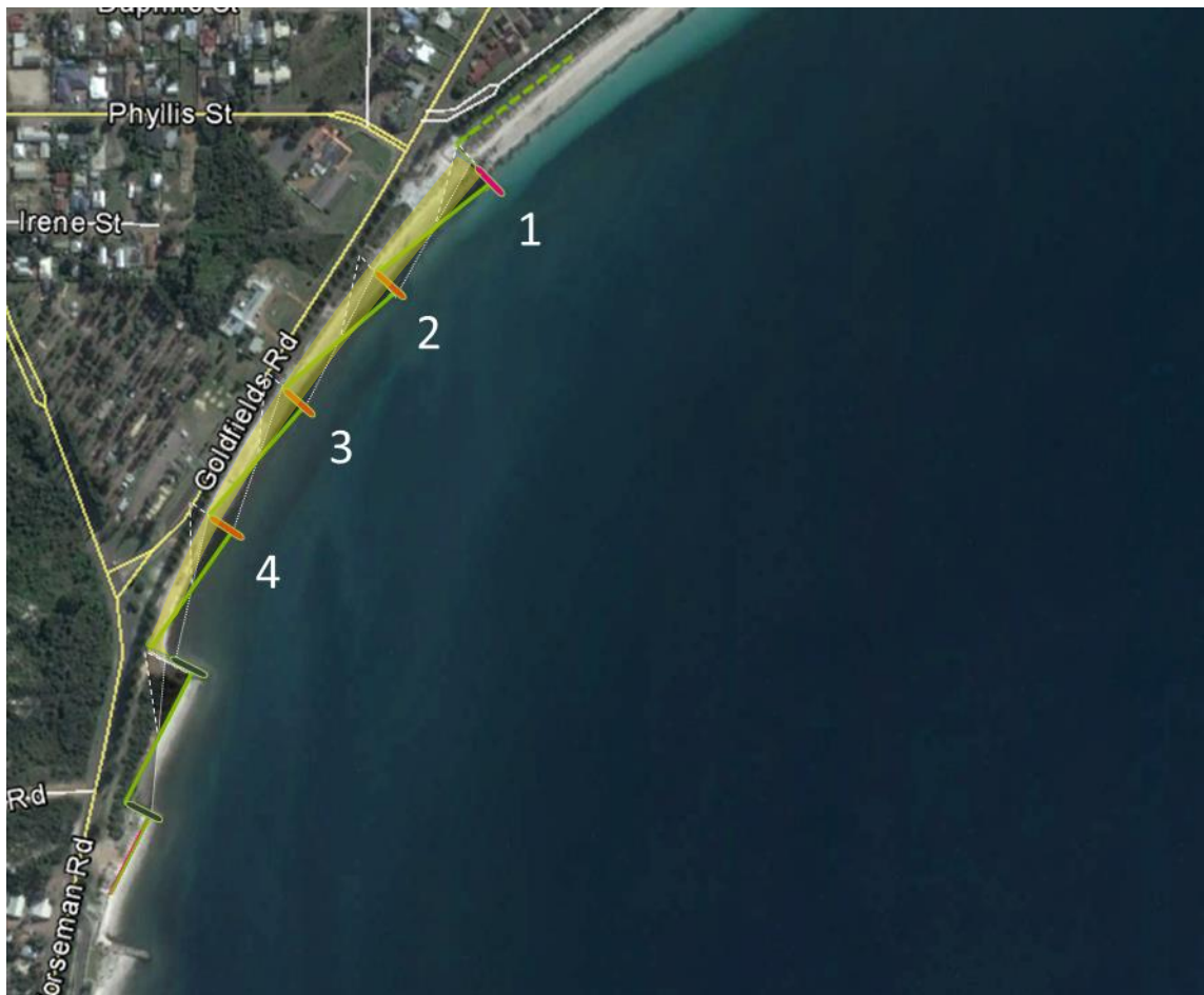
Figure 3-10: Illustration of Option 5 – Groyne(s) – 4 short groynes.
