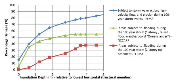
Figure 5-17: Inundation depth versus building damage curves (after FEMA<sup>iv</sup> and NCCARF<sup>v</sup>).
