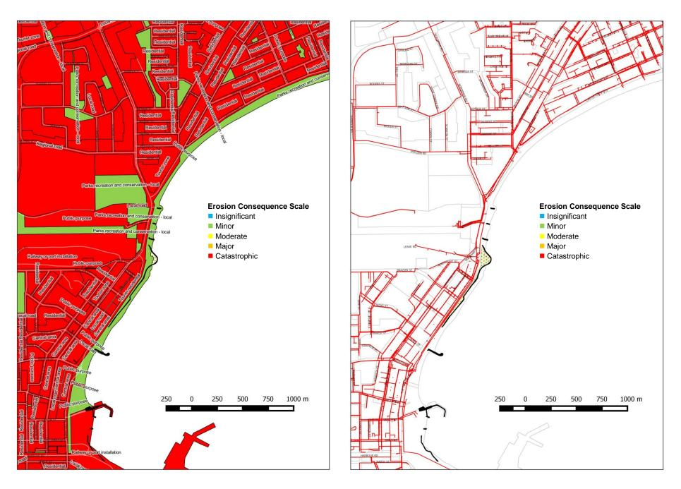
Figure 5-8: Erosion consequence for zoning (left) and infrastructure (right).
