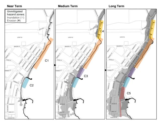
Figure 7-2: Protection scheme stages: C1: Construction of (existing) Esperance Seawall, C2: construction phase 2, C3: construction phase 3, C4: construction phase 4, C5: construction phase 5.
