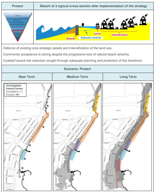
Protective structures ( $\blacksquare$ , $\blacksquare$ , $\blacksquare$ , $\blacksquare$ , $\blacksquare$ , $\blacksquare$ ) are added and maintained along the foreshore progressively in repsonse to the erosion of foreshore reserve at key trigger points locations ( $\star$ ). Inundation controls measures are integrated to the protection scheme.
