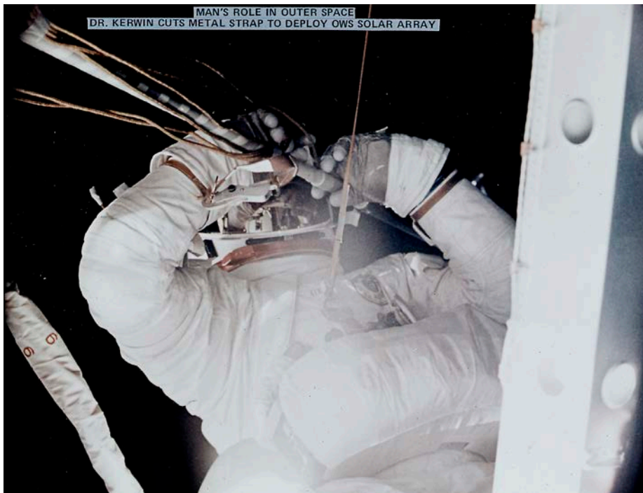
Left: This image shows astronaut Kerwin cutting the metal strap to free and deploy the Orbital Workshop solar array. Kerwin used special cutting tools developed by engineers at the Marshall Space Flight Center (MSFC). The MSFC had a major role in developing the procedures to repair the damaged Skylab. Credit: NASA
