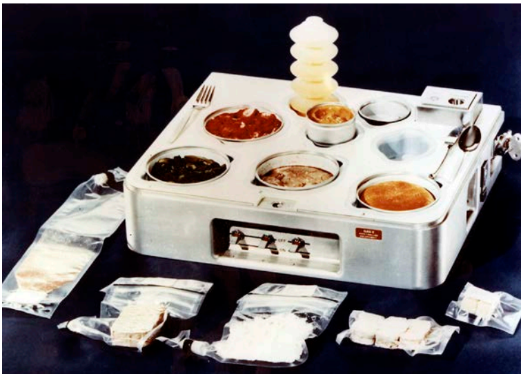
Shown here is the Skylab food heating and serving tray with food, drink, and utensils. The tray contained heating elements for preparing the individual food packets. The food on Skylab was a great improvement over that on earlier spaceflights. It was no longer necessary to squeeze liquified food from plastic tubes. Skylab's kitchen in the Orbital Workshop wardroom was so equipped that each crewman could select his own menu and prepare it to his own taste. Credit: NASA
